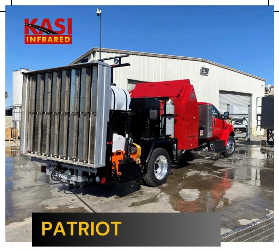
Truck mounted, self-contained IR restoration system.
