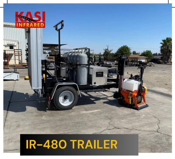
The Kasi IR-480 utilizes infrared radiation to heat existing asphalt pavement.
