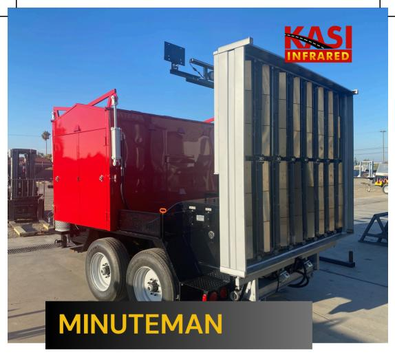
Trailer mounted 3-ton capacity asphalt reclaimer with a 48 square foot infrared heater.
