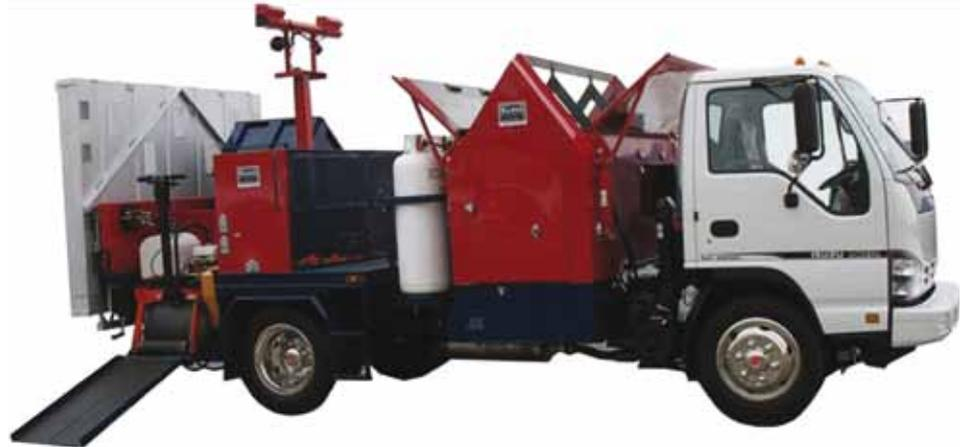
trailer-mounted Kasi Proheat 2 Ton Minuteman model, which is a self-contained asphalt restoration system. It is ideal for permanently repairing all general asphalt defects including potholes, surface cracking, utility cuts, trenches, birdbaths and manholes.
